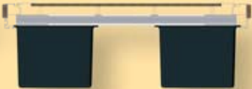
The floats can be changed without disassembling the dock. They are inserted in the profile on one side and blocked by bolts on the other. They are mounted catamaran-style for optimal stability
