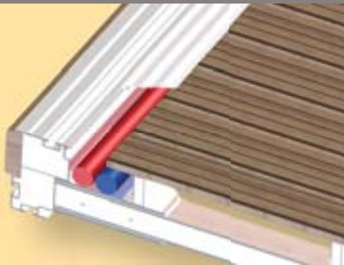
A specially designed profile covers utility channels to give fast, easy access to water and electricity systems
